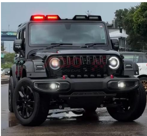
(Red-blue strobe lights fitted on the top, which produce quick, repeated, and extremely brilliant bursts of light in red and blue colours)
