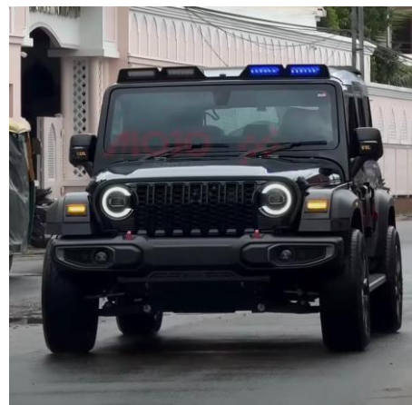
(Red-blue strobe lights fitted on the top, which produce quick, repeated, and extremely brilliant bursts of light in red and blue colours)
